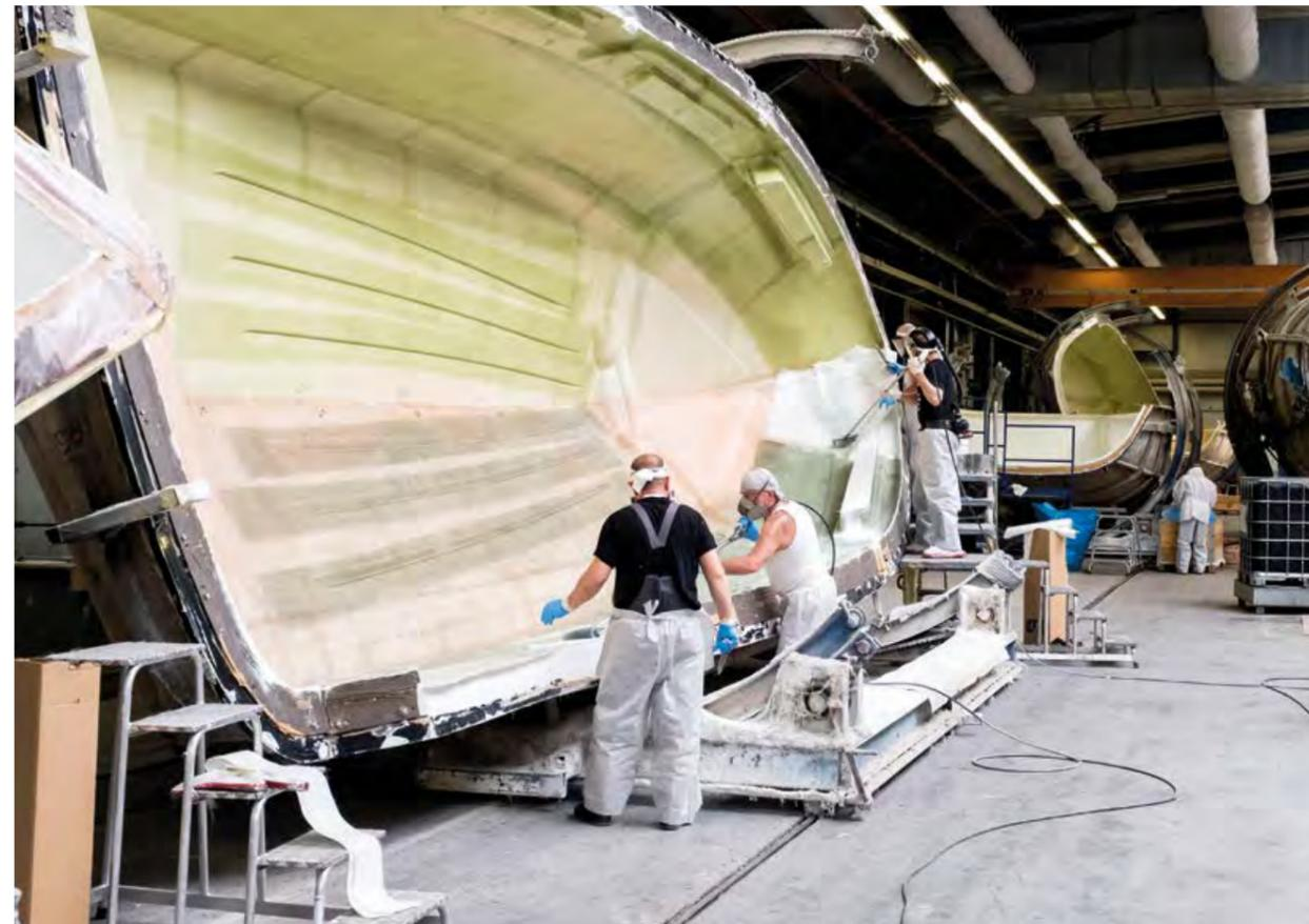
bow thrusters, and in the case of sailing yachts, the engines are also installed here. In some places on the inside, the surface is already sealed here with topcoat: "It's all about ensuring quality," says Christopher Marschka. And on the hulls and decks are already checked at this point for any blemishes in the gelcoat finish. These are much easier and more effective to touch up here than later on the assembly line.
